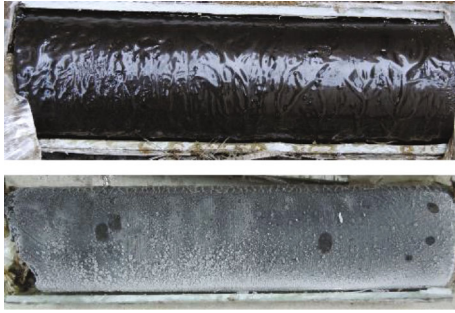
FIGURE 1: Oil sand core at room temperature and in a frozen state.
