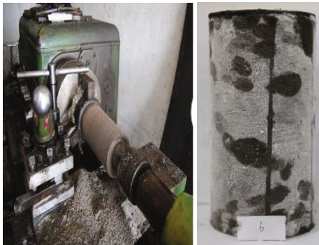
FIGURE 2: Oil sand core test specimen preparation process by lathe and the processed test specimen.
