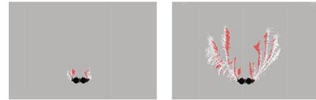
FIGURE 20: Acoustic emission damage cloud of 350-mm double hole.
