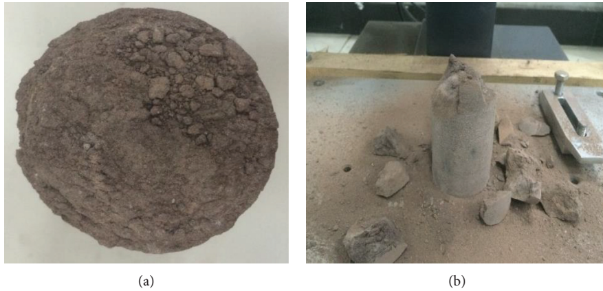
FIGURE 6: Failure observation of rock specimen after ultrasonic vibration. (a) Upper crushing of specimen (b) Large fragments separated from the body of the specimen.
