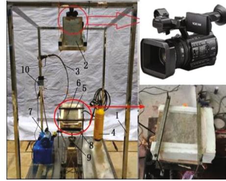
FIGURE 3: Diagram of the visual test device for fracture seepage. Picture of the experimental device. 1, test framework; 2, high-speed camera; 3, high-pressure pipe; 4, gas cylinder; 5, antifoam frame; 6, transparent resin; 7, motor test pump; 8, pressurized air cushion; 9, angle-adjusting instrument; 10, flow meter.
