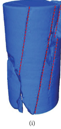
FIGURE 4: Failure modes of selected samples after uniaxial compression: (a) A-1; (b) A-2; (c) A-3; (d) B-1; (e) B-2; (f) B-3; (g) C-1; (h) C-2; (i) C-3. The dotted line represents the approximate position of the main fracture surface of specimens.
