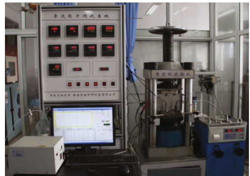
FIGURE 2: Fracture conductivity testing and analysis system.
