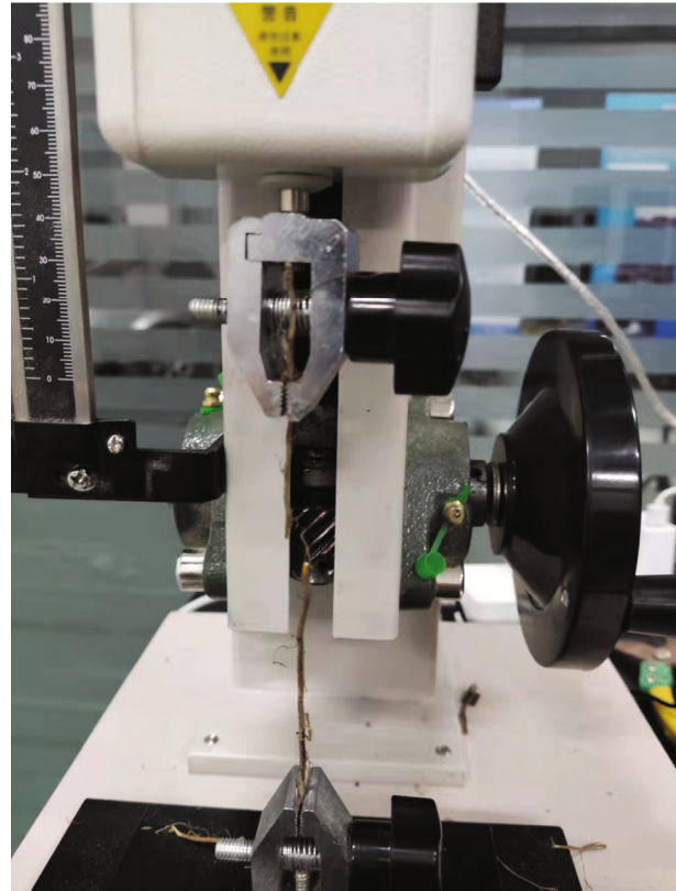
(b) Pull out test of A. fruticosa root
