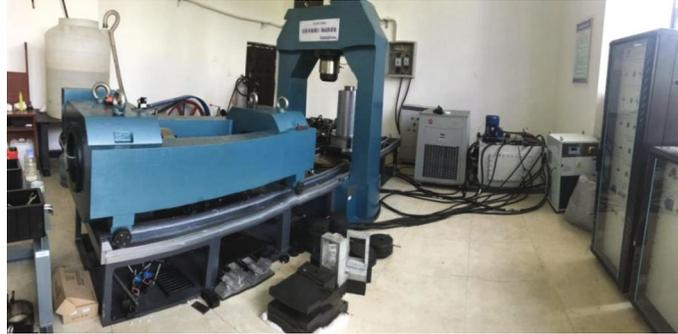
FIGURE 2: Rock joint shear-flow coupling test system.
