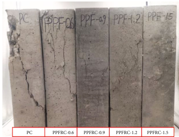
FIGURE 16: Uniaxial compression failure morphology of specimens at 28 days of curing age (sample 1).
