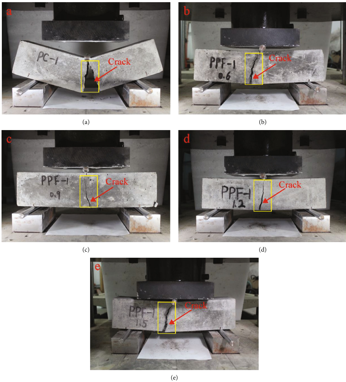
FIGURE 23: PC and PPFRC failure type: (a) PC (brittle) and (b-e) PPFRC (ductile).
