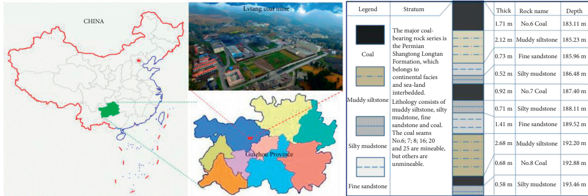
FIGURE 8: Geographical location of the Lvtang coal mine and the coal seam stratigraphic column.
