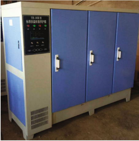
FIGURE 1: Alkali aggregate reaction curing box.
