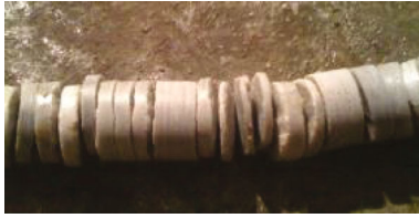
FIGURE 11: Borehole core after slotting.
