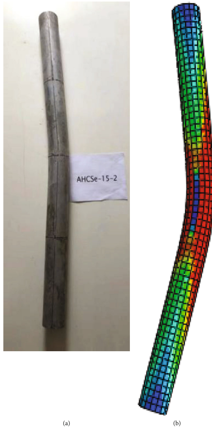
FIGURE 11: (a) Test failure mode. (b) Numerical analysis of failure mode.
