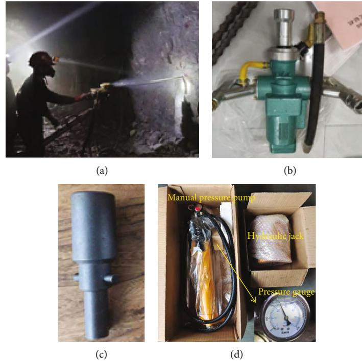
FIGURE 3: Test equipment. (a) Rock drilling. (b) Air-coal drill. (c) Mixing head. (d) Pulling equipment.
