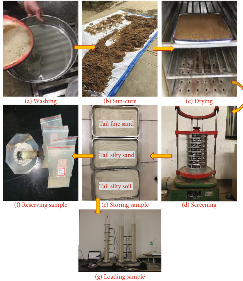
FIGURE 4: Preparation process of tailing sample.
