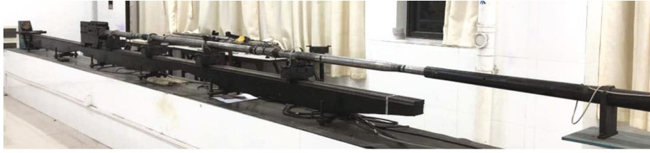
FIGURE 3: SHPB test device with variable cross section of 74 mm diameter.
