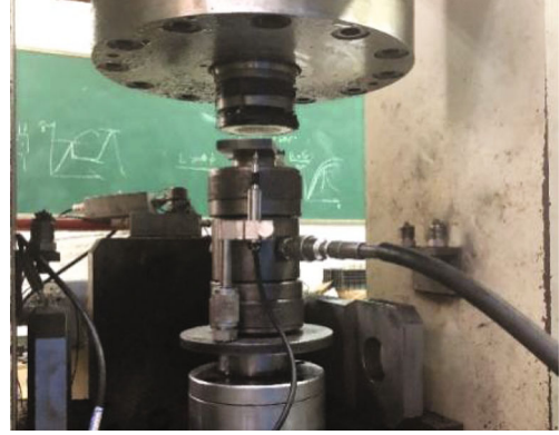
FIGURE 1: Conventional triaxial compression test.
