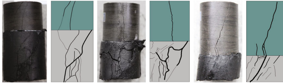
FIGURE 11: Crack propagation during loading of the coal-rock combined body.
