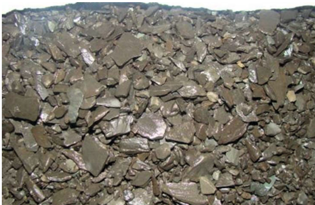
FIGURE 7: Debris from the middle-deep transition shale interval of Bohai oil field of China.
