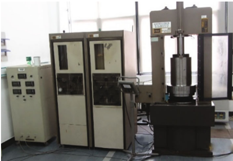
FIGURE 2: The 815.02 electro-hydraulic servo-controlled rock mechanics testing system.
