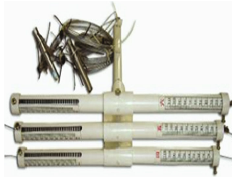
(a) DW-6 multipoint displacement meter
