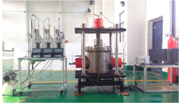
FIGURE 1: Physical diagram of gas-solid coupling coal seepage test system.
