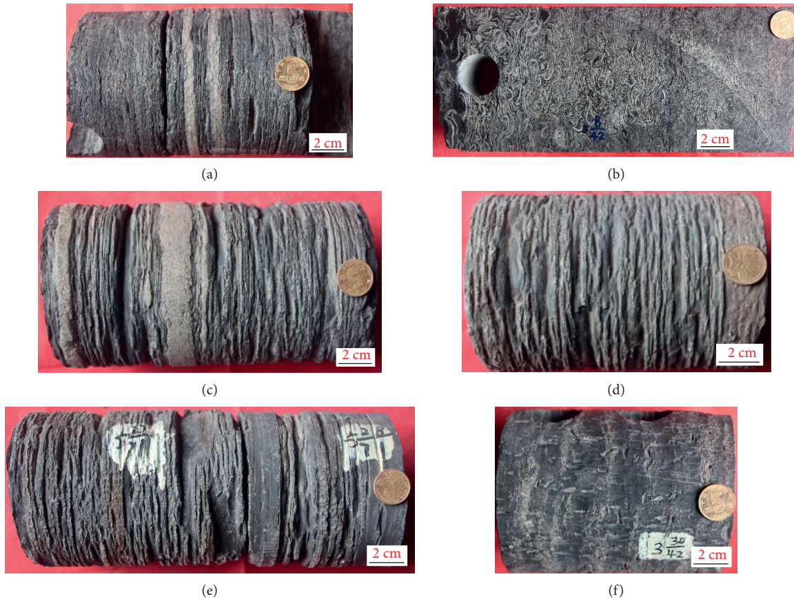
FIGURE 3: The lithology and laminar fracture of the fine-grained rock core of the Da'anzhai Member in the Sichuan Basin. (a) Shell limestone, shale intercalated with shale, lamina fractures developed, 1 North-1 Well, 3755.3 m. (b) Argillaceous shell limestone, shells arranged along the lamina, East-2 Well, 2152.5 m. (c) Intercalated limestone of gray-black shale, East-1 Well, 2618.23 m. (d) Black shale, laminar, and laminar fractures, East-1 Well, 2620.45 m. (e) Black shale, laminar and laminar fractures, East-1 Well, 2623.12 m. (f) Lime mudstone, East-2 Well, 2156.34 m.
