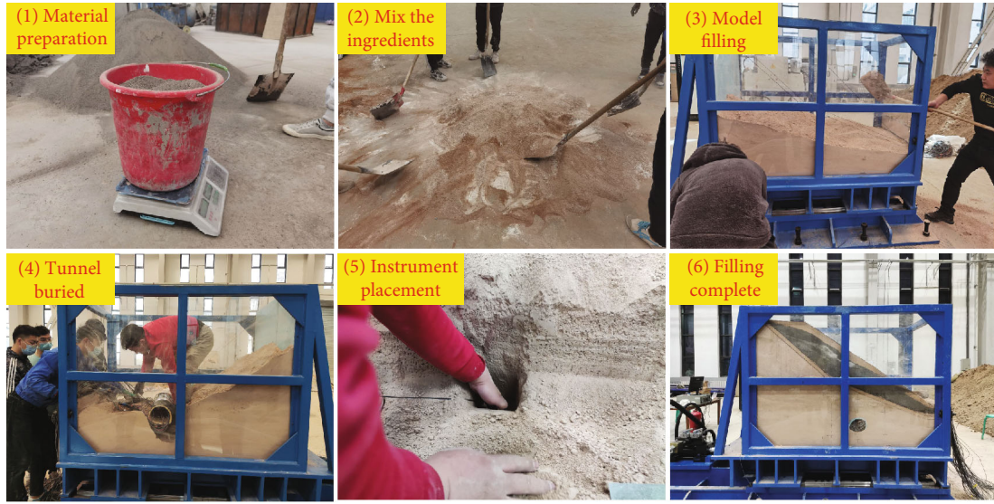
FIGURE 5: Shaking table model filling process.
