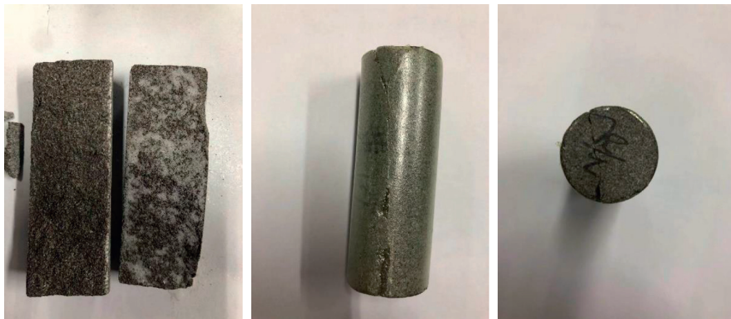
FIGURE 2: Artificial fractured core.
