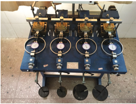
FIGURE 2: Strain controlled direct shear apparatus.
