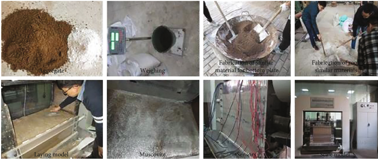
FIGURE 7: The construction process of the physical model.
