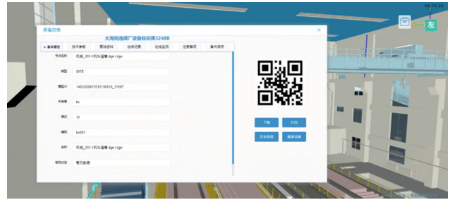
FIGURE 8: QR code management for equipment of Wangjialing Coal Preparation Plant.
