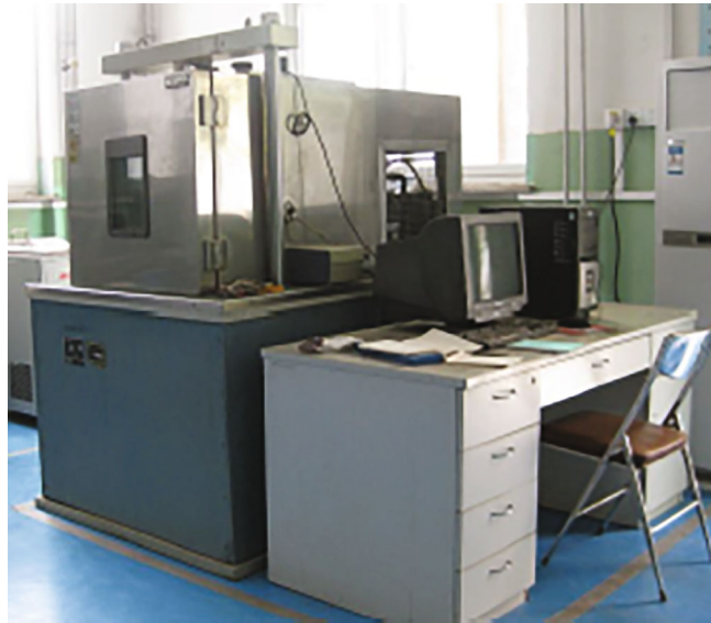
FIGURE 1: Unconfined compressive strength testing machine for frozen soil.
