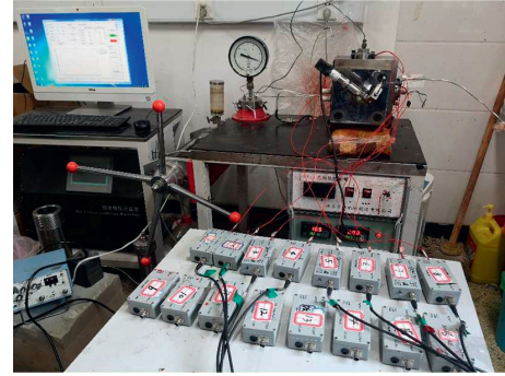
FIGURE 4: Small-size triaxial fracturing simulation system.
