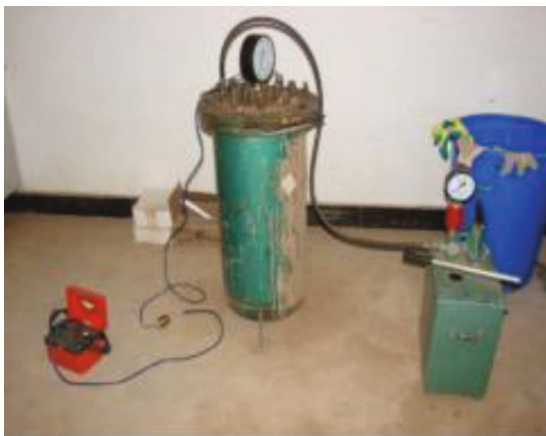
FIGURE 5: Sealing the pressure tank and pressurizing it.
