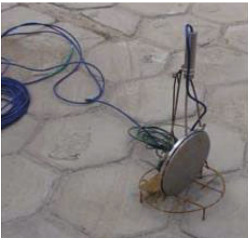
FIGURE 8: The fixing of soil pressure gauge.
