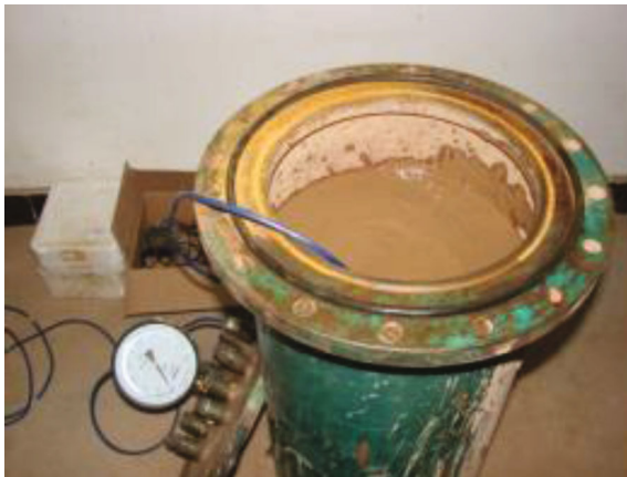
FIGURE 4: Muddy water is injected into the pressure tank.
