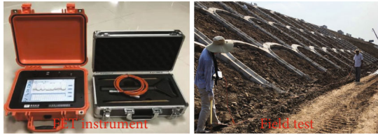
FIGURE 15: FET audiofrequency magnetotelluric instrument and field test.
