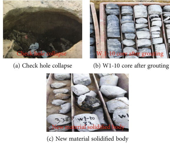
FIGURE 14: Drilling detection of grouting effect.
