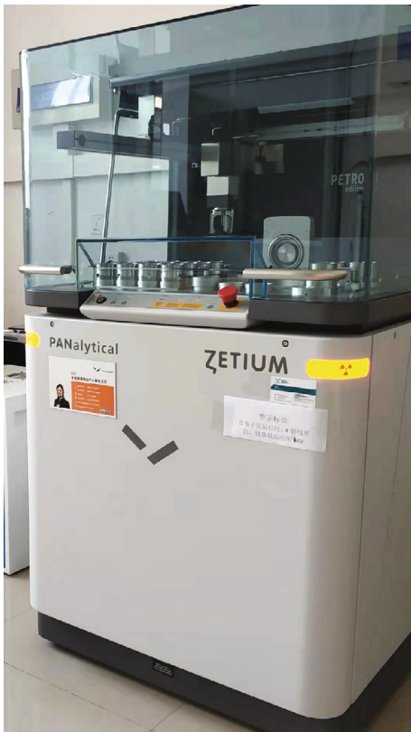
FIGURE 2: XRF test system.
