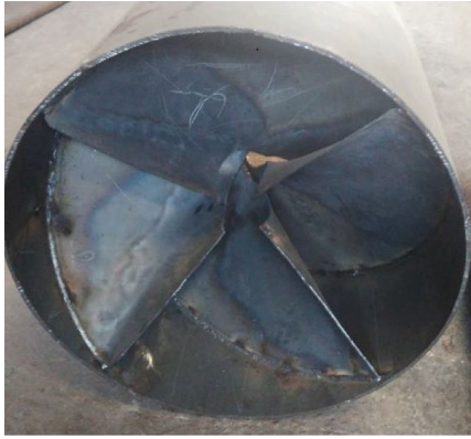
FIGURE 19: Arrangement of spiral blades in the experimental unit.
