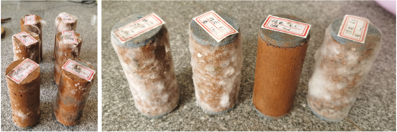
FIGURE 3: Sample of silty clay containing crushed stone after curing for 28 d.
