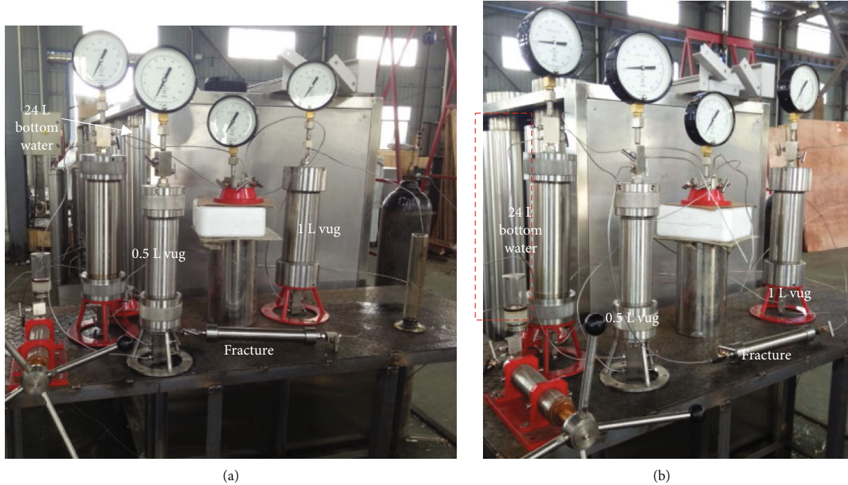
FIGURE 2: Pictures of high-pressure physical simulation experiment model for (a) bottom water connected to the large vug and (b) bottom water connected to the small vug.
