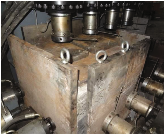
FIGURE 14: The horizontal loading way bearing plate.
