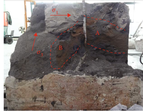
FIGURE 16: The hydraulic fracturing morphology of turning test: (A) surface 1; (B) surface 2.
