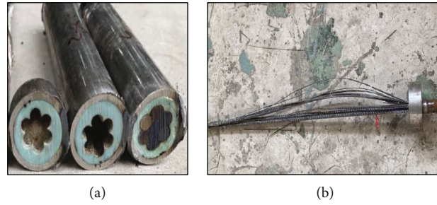
FIGURE 3: The failure mode of the “BFRP-connector-strand.” (a) Steel strand pulled out from the steel connector; (b) BFRP tendon rupture.
