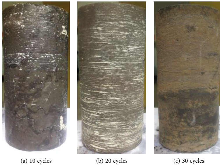
FIGURE 9: Change of appearance characteristics of some specimens after cyclic immersion.
