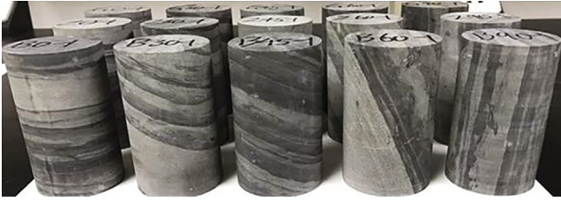
FIGURE 1: Schematic diagram of uniaxial compression samples of carbonaceous slate with different bedding inclination angles.
