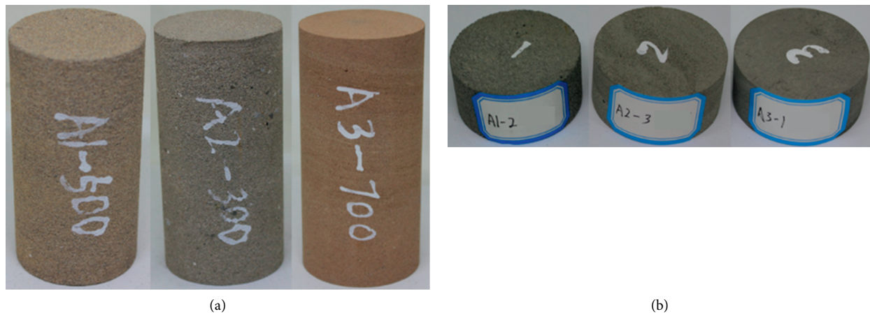
FIGURE 4: Uniaxial compression/Brazilian splitting test specimens. (a) 50 * 100 mm uniaxial compression test specimens (b) 25 * 50 mm Brazilian splitting test specimens.
