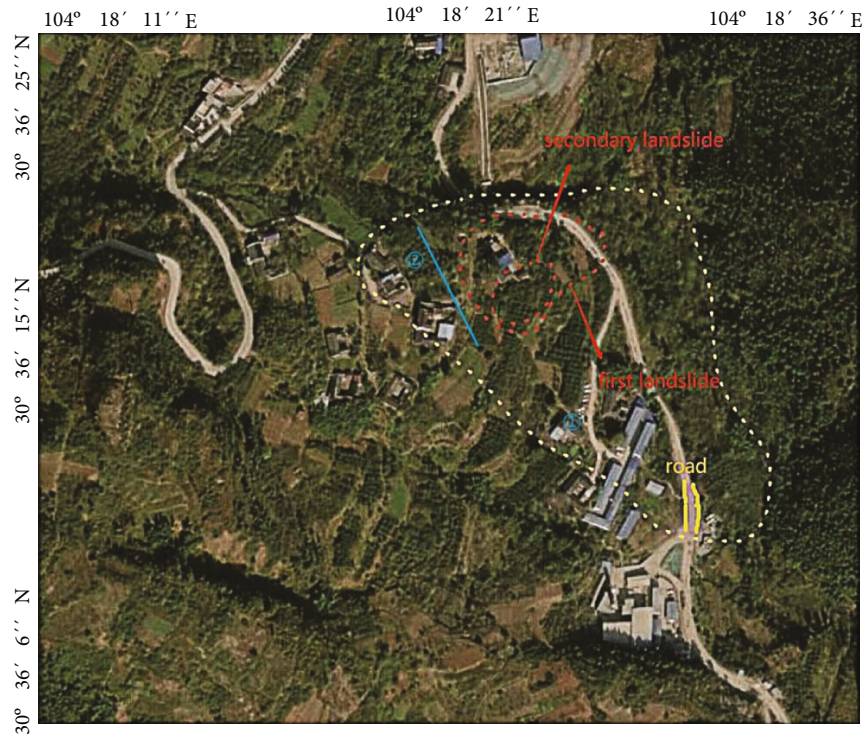
FIGURE 5: Satellite image before the landslide. The red dotted line indicates the area of the first landslide and the second landslide. The yellow dotted line indicates the entire study area.
