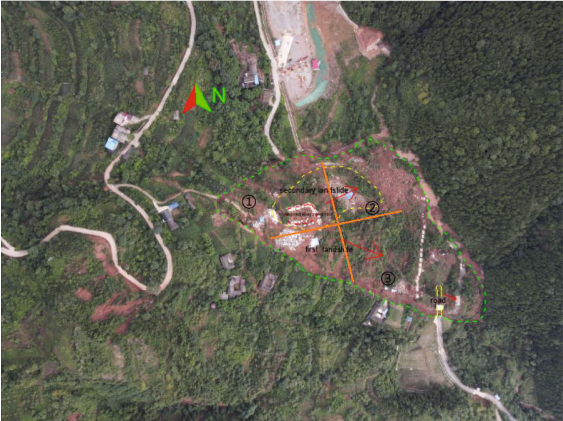
FIGURE 3: Aerial photo taken by drone. The yellow dotted line indicates the secondary landslide caused by pool collapse, and the red arrow indicates the sliding direction of landslide.
