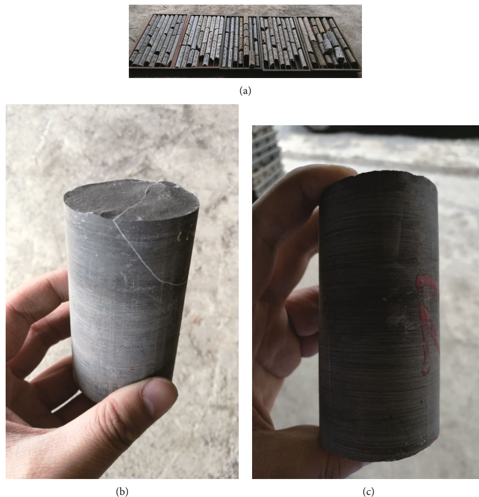
FIGURE 1: Deep rock samples. (a) Drilled rock sample. (b) Limestone sample. (c) Silty mudstone sample.
