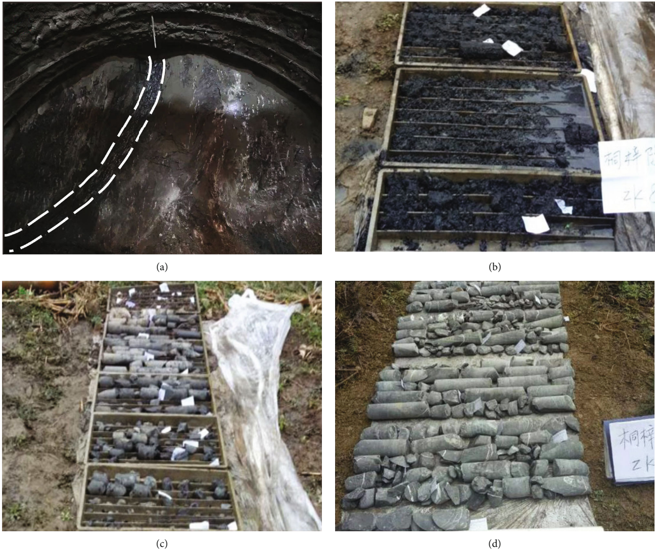
FIGURE 3: Stratigraphic samples. (a) Coal seam on the tunnel face. (b) Coal seam. (c) Limestone intercalated with mudstone. (d) Mudstone.
