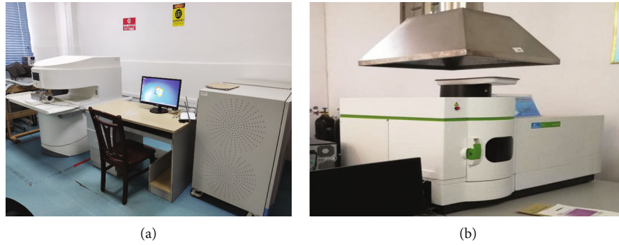
FIGURE 2: Test equipment. (a) Large aperture NMR imaging analyzer. (b) Inductively coupled plasma atomic emission spectrometer.
