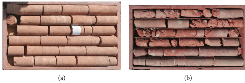
FIGURE 3: Rock cores drilled in the Yingpanhao mine of (a) Cretaceous strata and (b) the Jurassic Anding Formation.
