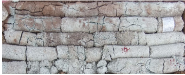
FIGURE 8: Disintegration of Jurassic sandstone core after encountering water.
