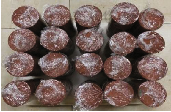
FIGURE 3: Indoor environment, cling film wrapped specimen watering maintenance.
