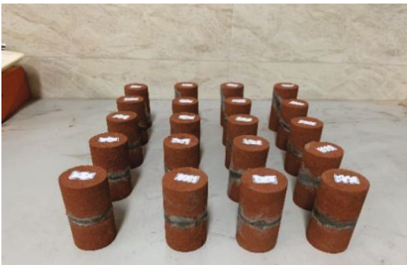
FIGURE 4: Red sandstone crack grouted body specimens.
