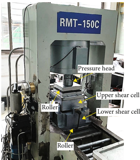
FIGURE 5: Direct shear test by RMT-150C servo test system.
