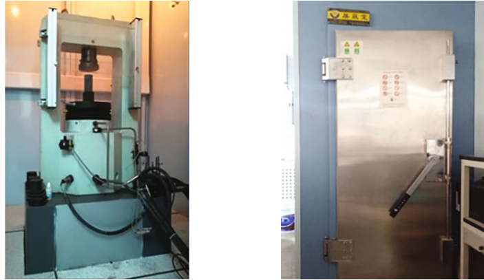
(a) YAW-600 microcomputer-controlled loading system (b) EMR shielding room
