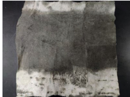
(a) Tailing sand residue in geotextile
