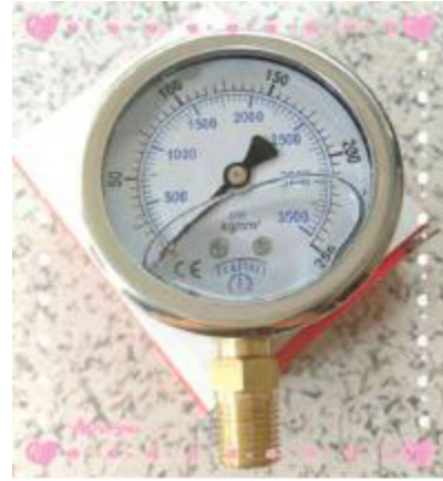
FIGURE 5: The photograph of oil pressure gauge.
