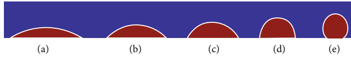
FIGURE 6: Droplet shape at different contact angles: (a) \theta = 30^\circ , (b) \theta = 45^\circ , (c) \theta = 60^\circ , (d) \theta = 90^\circ , and (e) \theta = 135^\circ .
